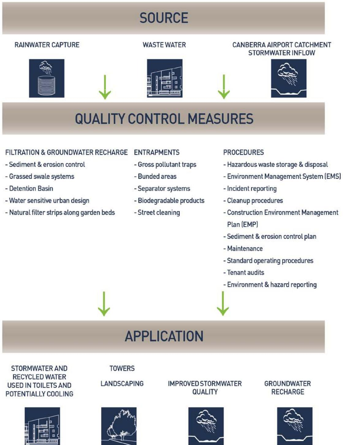
Figure 2: Canberra Airport water recycling and reuse
